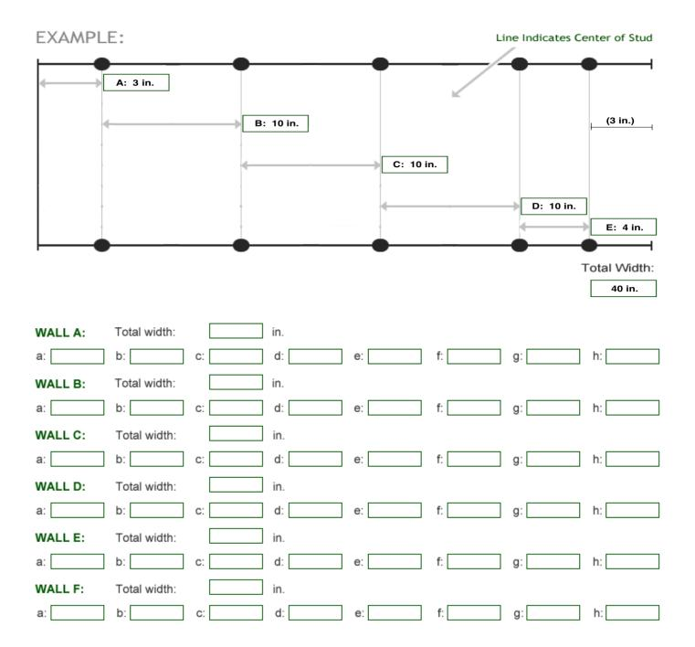
Assessing the width of the pads consists of two very important measurements. First, **measure the total width of the cab wall that the pad is to cover**. This is the total width of the wall and the corresponding pad that will cover it.
