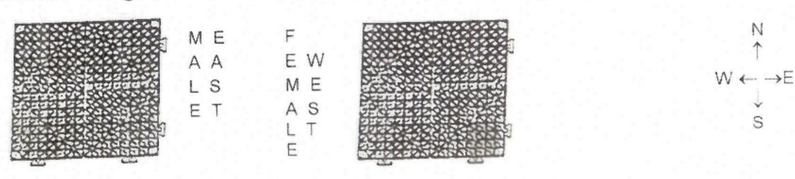
For the second row - go back to the first tile that you put down. Take a tile and put the female (north side) of the tile down on top of the male tab (south side) of the first tile. Continue doing this until you have completed the second row.
