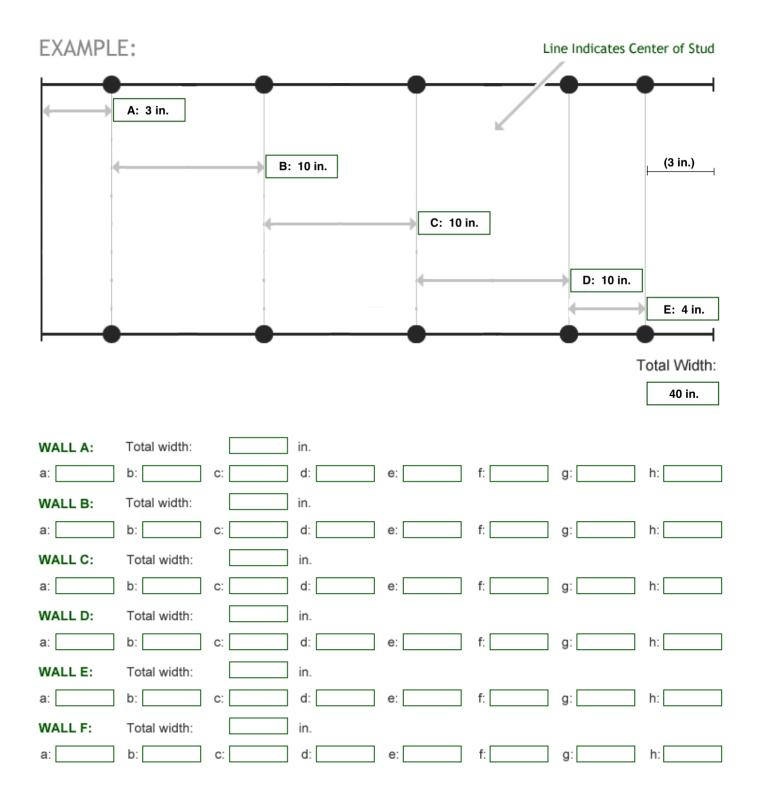
Assessing the width of the pads consists of two very important measurements. First, **measure the width of the cab wall that the pad is to cover**. This is the total width of the wall and the corresponding pad that will cover it.
